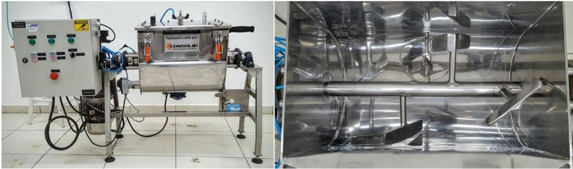
**Figure 2.3.** Intensive Horizontal Mixer Consolid. (a) external view, (b) internal view
